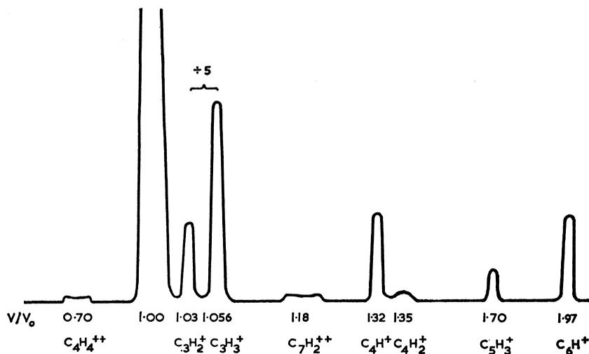
Fig. 2. Precursor ions of the  $C_3H^+$  product ion in the mass spectrum of toluene obtained on an MS9 instrument by scanning the accelerating voltage,  $V$ , at constant  $E$  and  $B$ . (Reproduced with permission from K.R. Jennings, *Some Aspects of Metastable Transitions*, in G.W.A Milne (Ed.), *Techniques and Applications*, John Wiley and Sons, Inc., New York, 1971, p. 419.)
