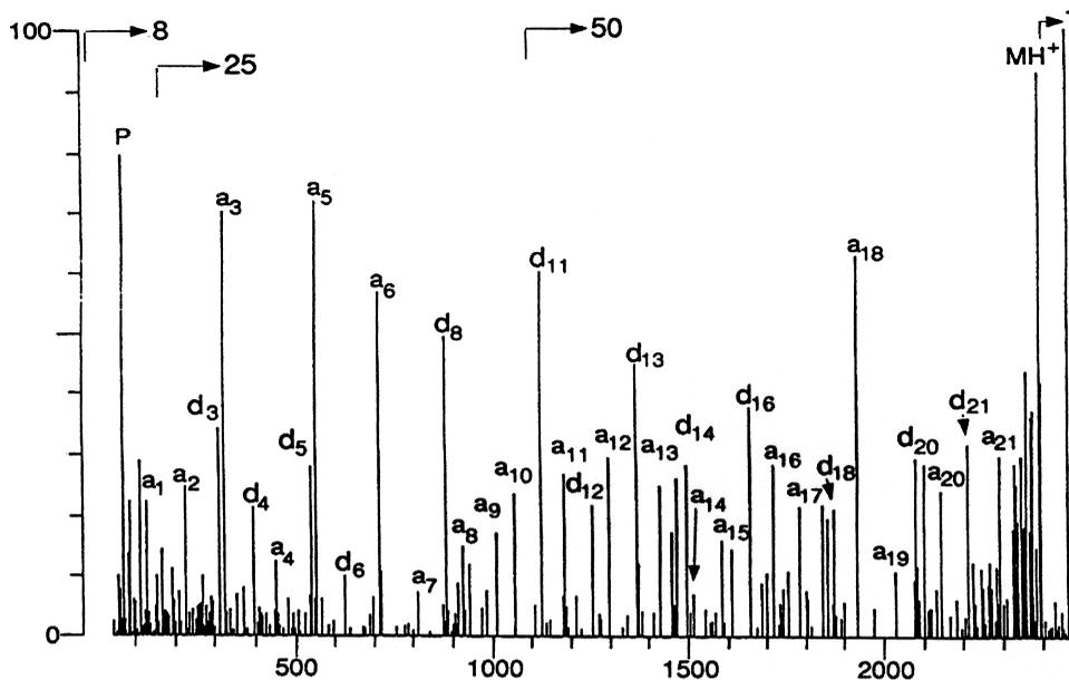
Fig. 3. A CID spectrum obtained by use of a four-sector instrument to sequence the peptide CLIP,  $m/z$  2465, with argon as collision gas, showing a complete sequence of *a* ions yielding the sequence RPKVKVYPNGAEDESAEAFPLEF.
