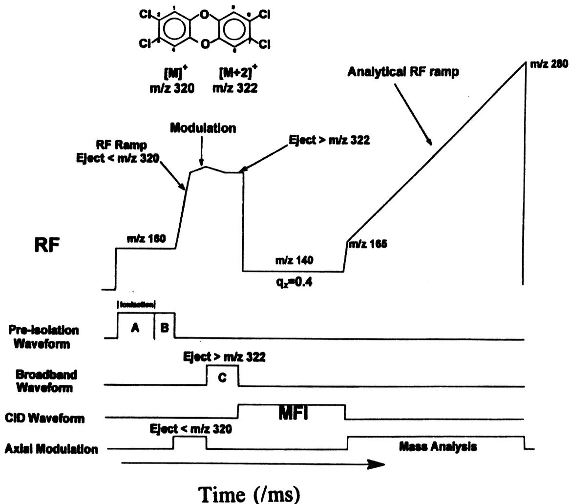
Fig. 5. Scan function for the CID of the  $m/z$  320 and 322 molecular ions of dioxin in an ion trap. (Reproduced with permission from Ref. 48.)
