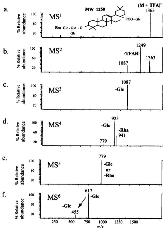
Fig. 7. The  $(MS)^6$  CID spectrum of oleanolic acid glycoconjugate (molecular weight 1250) obtained by means of an ion trap. (Reproduced with permission from Ref. 52.)
