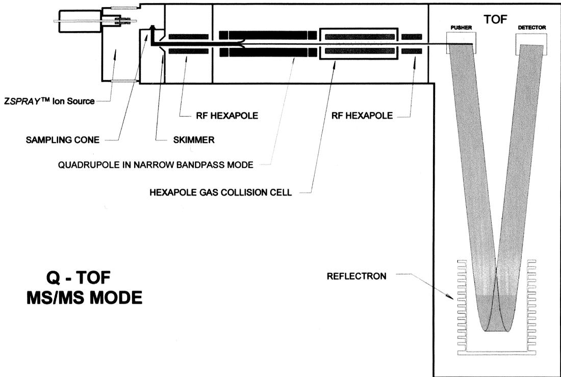
Fig. 4. Schematic of the Micromass Q-TOF tandem mass spectrometer. (Courtesy of Micromass UK Ltd.)
