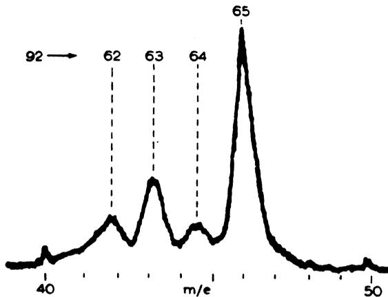
Fig. 1. Part of the CID spectrum of the toluene molecular ion observed in an MS9 double-focusing magnetic sector instrument. (Reproduced from Ref. 4.)
