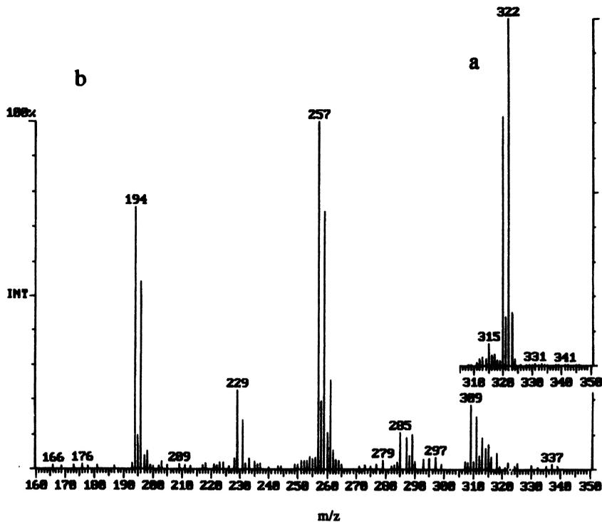
Fig. 6. Ion trap spectra (a) showing the isolation of the  $m/z$  320 and 322 molecular ions of dioxin and (b) showing the CID spectrum of these ions. (Reproduced with permission from Ref. 48.)
